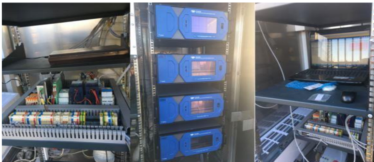
Photo 2: Data logger, parameters for measurement of air quality and PC/laptop (for collection of generated data)
